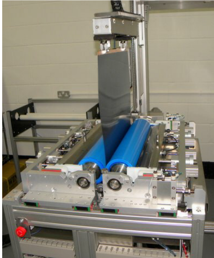
Phot.2 Double-sided grooved-roller resist coater.
