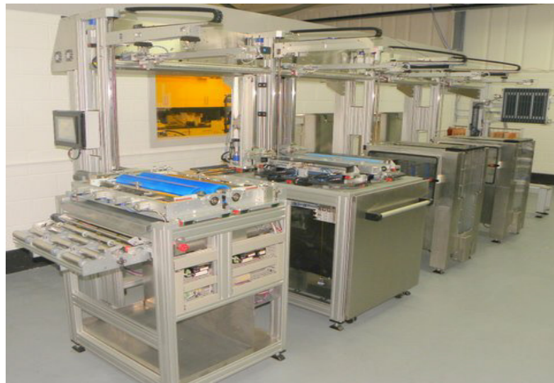
Phot 1 Complete Rainbow demonstration line without its clean air enclosure.
