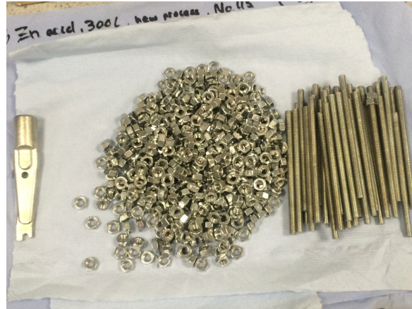
Fig.2: Improved zinc plating on cast items and fixings using ultrasound.
