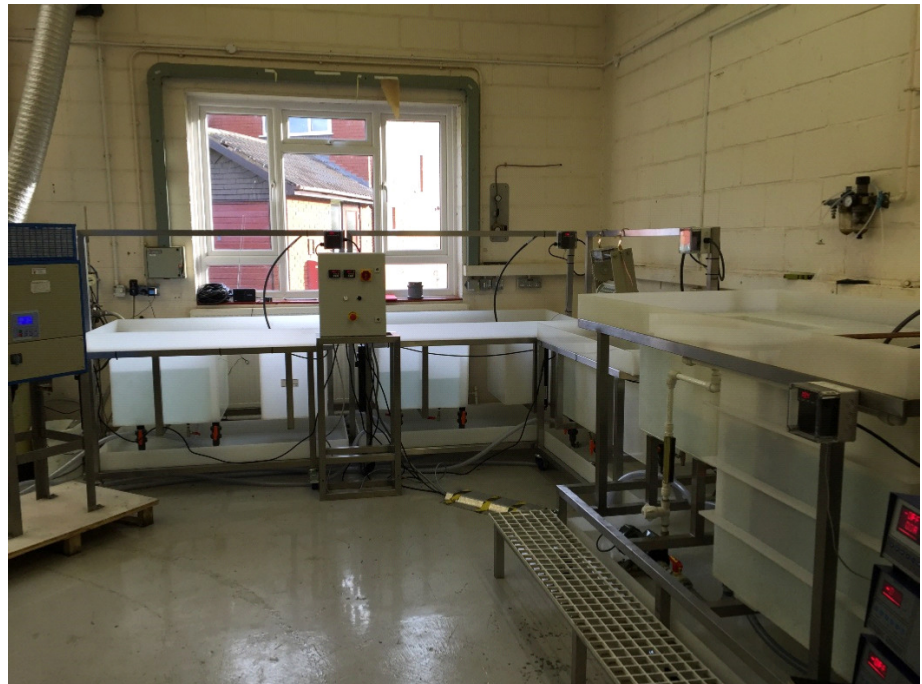
Fig.1: Plating line at C-Tech incorporating ultrasound equipment.
