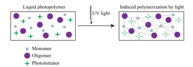
Acrylate – free radical cure Epoxy – cationic cure Hybrid – combination epoxy/acrylate system
